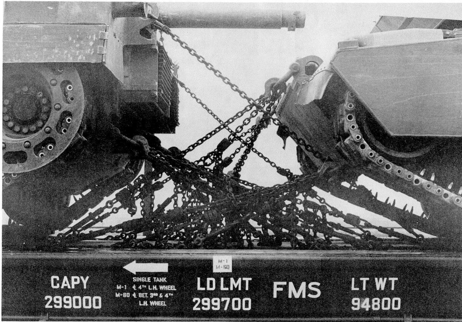
Figure 4-6. Between-tanks arrangement of chain tiedown devices.
